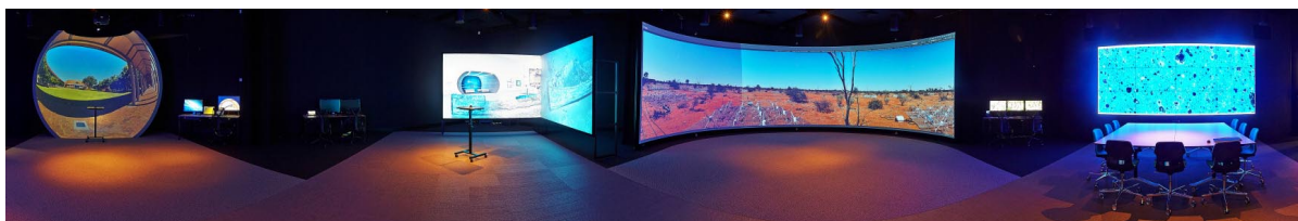
Figure 5. 360° image of the Curtin University HIVE (Hub for Immersive Visualisation and eResearch) visualisation facility. It houses four large-scale immersive displays: (a) Dome - four-metre diameter domed screen; (b) Wedge - two rear-projected 3.8m diagonal display in a 90° wedge configuration; (c) Cylinder - 3m high 8m diameter cylindrical projection display; and (d) Tiled - 12 x 55" Full HD displays.
