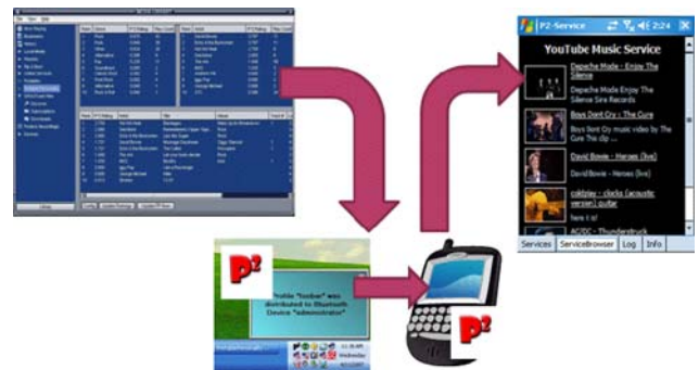
Fig. 13 Screenshot of the different P2 components in use for the audio-visual content scenario, where the profile is exchanged via Bluetooth
