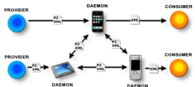
Fig. 4 Overview of the P2 system architecture with multiple provider and consumer nodes interconnected through the distributive P2 daemon network
